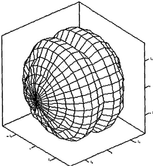
**Figure 18** 3D polar response (smoothed) of 0.3 m<sup>2</sup> DML panel, 8kHz
