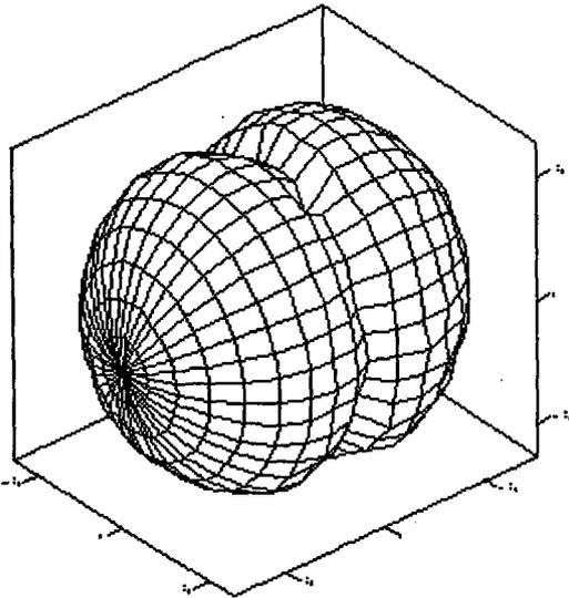
**Figure 17** 3D polar response (smoothed) of 0.3 m<sup>2</sup> DML panel, 300Hz
