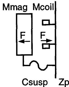
Figure 5 Mechanical arrangement for inertial drive DML panel
