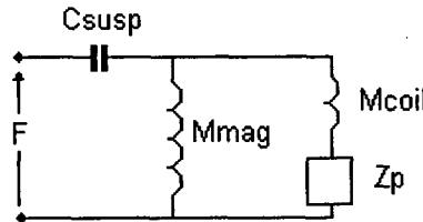
Figure 8 Electrical impedance analogue, with all transformers removed
