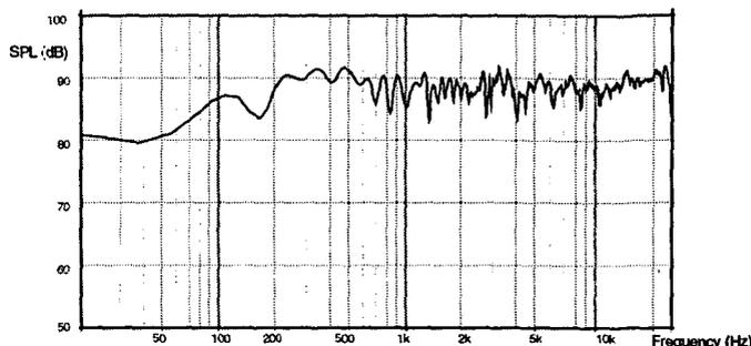
Figure 15 Typical unsmoothed frequency response of a DML panel
