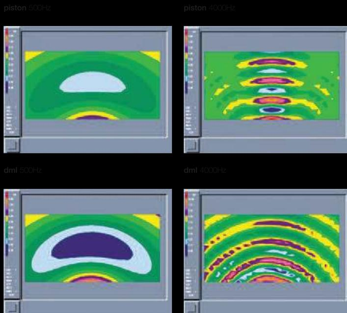
**figure 13** virtual image location in a two-channel stereo system is more accurate with distributed-mode sound sources
