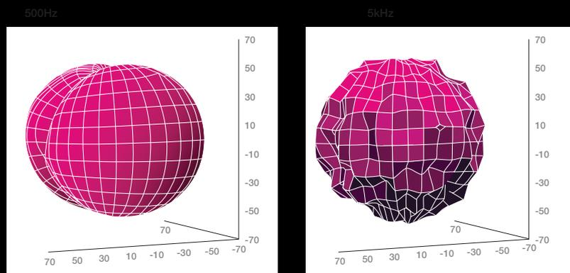
Although an NXT panel's vibrational behaviour appears random, the process of designing it is deterministic. Provided you know a few key parameters – the size and shape of the panel (it can be curved in one or more planes), the position of the exciters (the driving elements) and the bending stiffness, surface density and internal damping of the panel material – it is possible to predict the acoustic performance with
