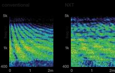
**figure 16** spatial correlation polar plots for an NXT panel and cone speaker illustrate the unique diffuse nature of the panel's sound radiation.
