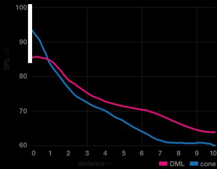
Because of the diffuse nature of a DML's acoustic output the correlation coefficient is much reduced off the reference axis, so room interaction is quelled.
