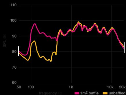
**figure 9** single-point sound pressure measurements display fine structure that is strongly dependent on the positioning of the microphone
