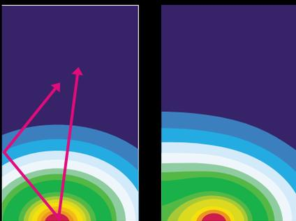
Because their diffuse acoustic radiation reduces destructive interaction with nearby reflective surfaces, free-standing NXT panels have no requirement for an enclosure. This eliminates the problems associated with loudspeaker cabinets, which have their own spurious resonances, colorations and cost penalties.
