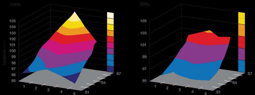
**figure 19** The diffuse radiation of an NXT panel improves acoustic feedback margin where speakers and microphones are in close proximity
