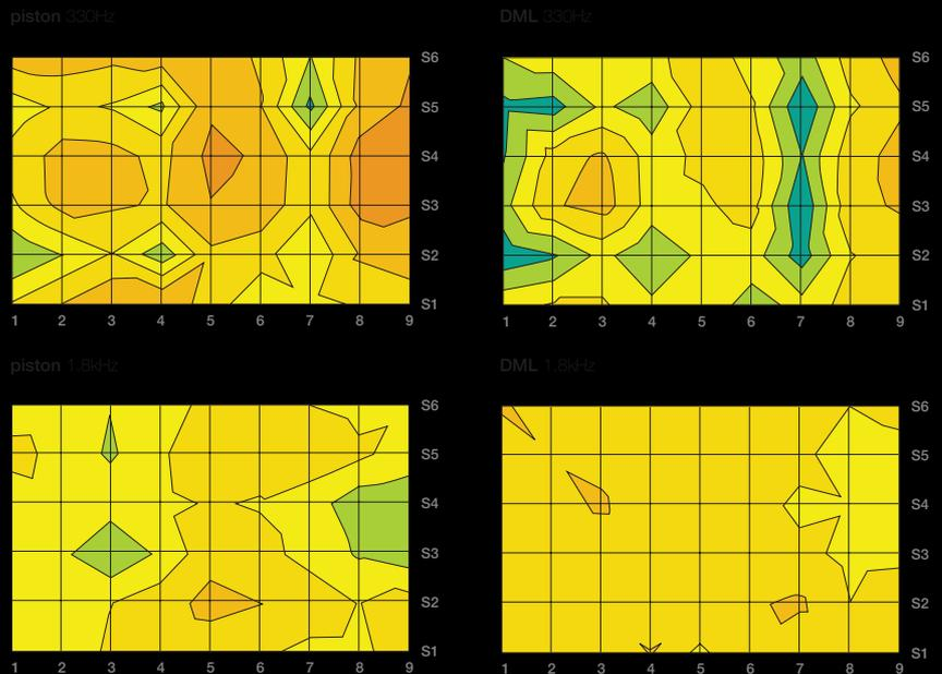
**figure 15** spectrograms of sound pressure level (false colour) versus frequency and distance confirm that an NXT panel interacts less destructively with a single boundary.
