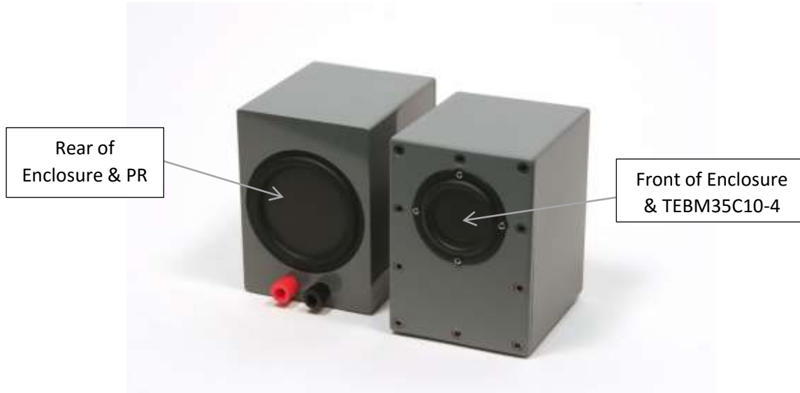
Figure 5. Outlook of 600 cc prototype. Outer/inner dimensions (WxHxD): 8.0 x 11.0 x 9.2 cm / 7.4 x 10.4 x 8.4 cm.
