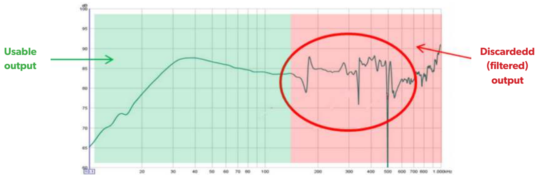
Figure 5. On-axis response of cone diaphragm speaker. Only part of the frequency range is usable, the region where breakup occurs (red) must be filtered away.
